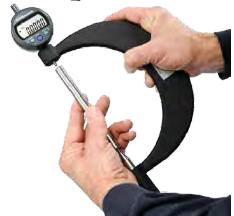
Setting PD-8001-RSC with Rod Standard
