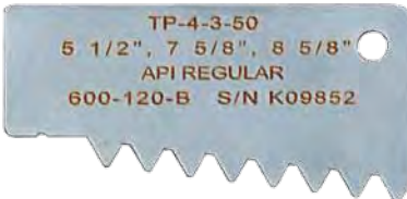
Assorted Tapered Thread Profiles
