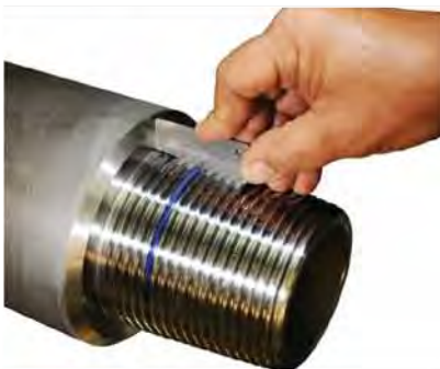
LPP on a Pin with blue line marking proper thread
