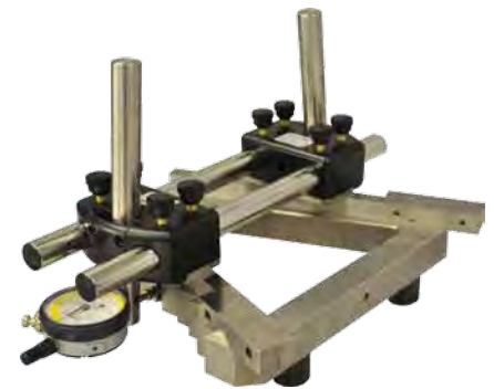
MRP-2000 on pin step standard
